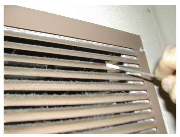
Collection of surface sample after 7 days of exposure to Air Naturalizer
